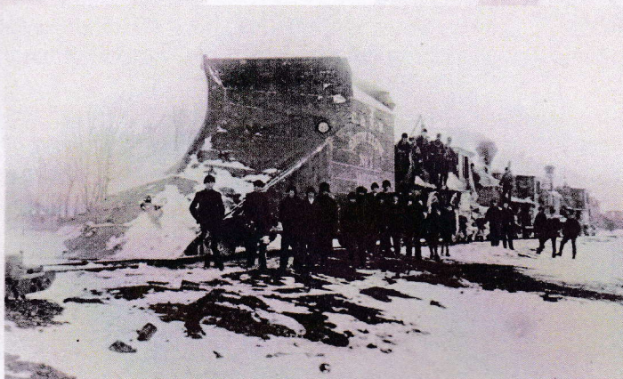
An unusual plow, built of wood, and significantly larger than the usual wedge plow. Note that this special implement sits in front of at least three locomotives. This photo was taken in Waseca, Minnesota, in 1880. Photo courtesy of the Chicago & North Western Historical Society.
